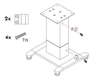
4 Attach top plate to the column with 6x M8 screws
